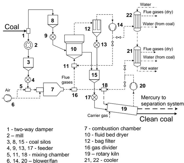
**Fig. 2.** Process diagram of a system for mercury removal from fuel using low-temperature pyrolysis.
