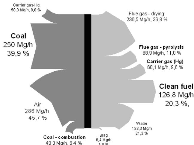
Fig. 4. Process mass balance of mercury removal from fuel using low-temperature pyrolysis; brown coal
