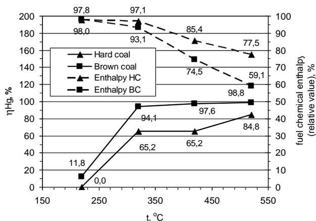
**Fig. 1.** Efficiency of Hg removal from hard (HC) and brown (BC) coal and relative value (to the raw coal) of chemical enthalpy of the fuel versus the process temperature
