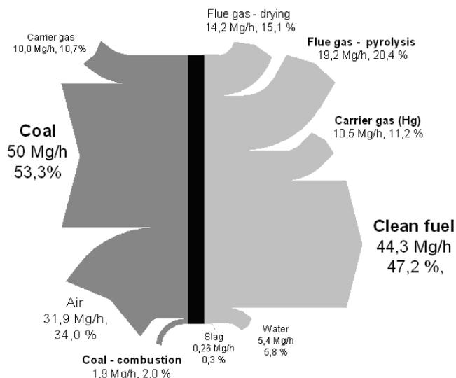
Fig. 3. Process mass balance of mercury removal from fuel using low-temperature pyrolysis; hard coal
