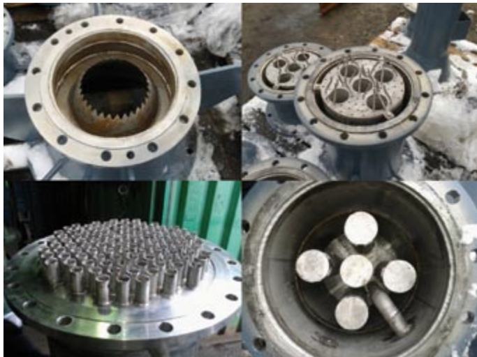
Fig. 6. Gas and liquid distributors in the absorption column
