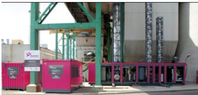
Fig. 7. Carbon capture mobile pilot plant during tests at the Łaziska Power Plant in Łaziska Górne, Poland
