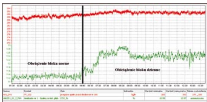
Fig. 11. \text{CO}_2 concentration fluctuations in the pilot plant flue gases (several hours)
