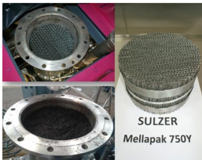
Fig. 5. Column structure packing and filters (activated carbon)
